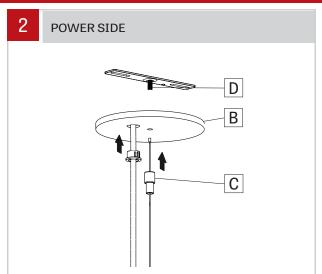
Secure canopy (B) with slip ring (C) on threaded rod (D). For a continuous system, please proceed to step 9.
