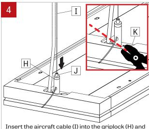
Insert the aircraft cable (I) into the griplock (H) and repeat on both sides of fixture. Adjust the cable (I) length by pushing the feeder tube (J) and **cut the excess cable** with an aircraft cable cutter (K).
