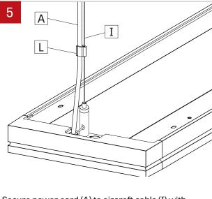
Secure power cord (A) to aircraft cable (I) with plastic clip (L).
