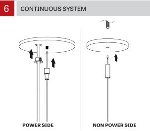
For a continuous system, repeat steps 1 to 3 for all mounting points. Repeat steps 4 and 8 for the first fixture.
