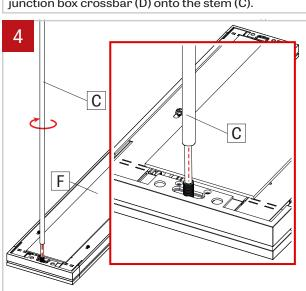
Screw the stems (C) onto the nipple at the ends of the fixture (F).
