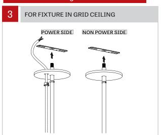
In the case where the luminaire is installed on a **grid ceiling**, the power cable will pass outside of the stem.
