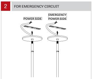
In the case where an **emergency circuit** is required, the wires to the emergency circuit will be passed through a second stem.
