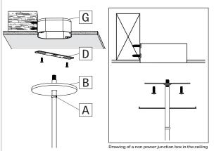
Raise the fixture and tighten the junction box crossbar (D) with screws (by others) to the junction box (G). Then slide the canopy (B) and thighten the set up with the slip ring (A).
