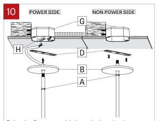
Raise the fixtures and tighten the junction box crossbars (D) with screws (by others) to the junction boxes (G). Make wire connection on the power side with wire connectors (H). Then slide the canopies (B) and thighten the sets up with the slip rings (A).
