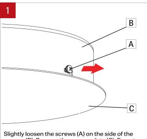
canopy (B). Remove the canopy plate (C). Do not completely remove the screws (A).
