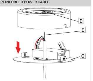
Release the cable (E) by pushing the feeder tube of the grip lock (D). Remove the canopy plate (C) .
