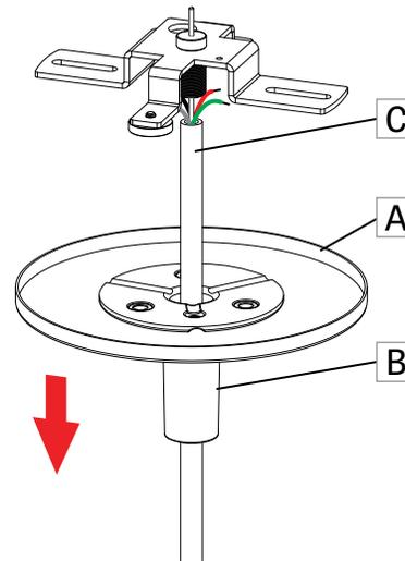
Lower the canopy (A) and the cone (B) along the reinforced cable (C).
