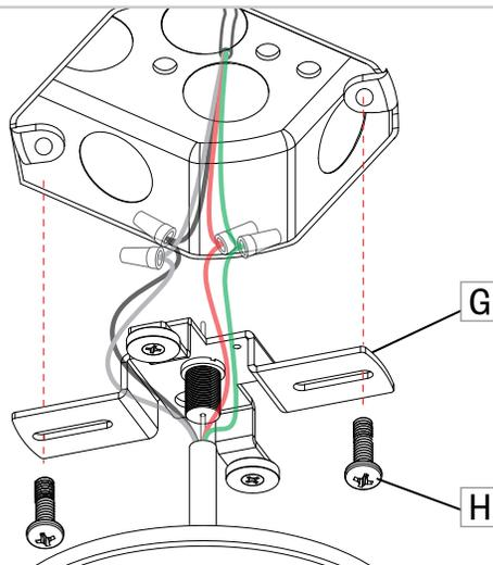
Install the cross-bracket (G) on the junction box with screws (H).
