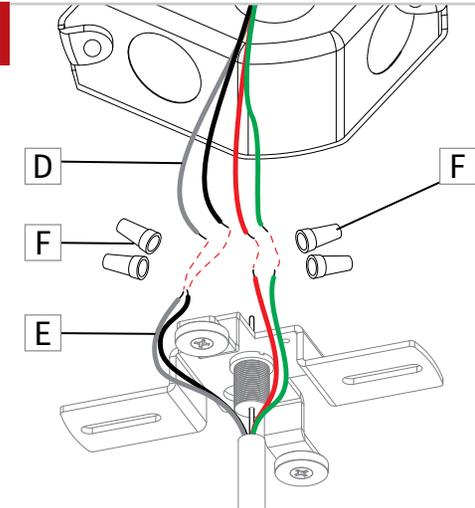
Make the electrical connection between the wires (D) from the building and the power cord (E) on the fixture with the marettes (F).
