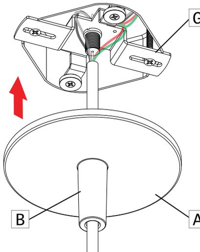
Attach the canopy (A) and the cone (B) on the magnetic cross-bracket (G).
