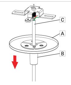
Lower the canopy (A) and the cone (B) along the reinforced cable (C).
