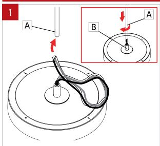
Pass the wires through the stem(A). Assemble the stem(A) into the cone(B) by screwing it.
