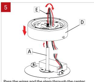
Pass the wires and the stem through the center hole of the canopy(D) and the nut(E). Drag back the wires through the canopy(D). Screw the nut(E) onto the stem(A).
