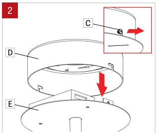
Slightly loosen the screws(C) on the side of the canopy(D). Remove the canopy plate(E). Do not completely remove the screws(C).
