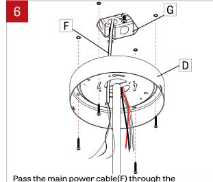
canopy(D). Fix the canopy to the junction box(G). Then, fasten the canopy(D) to the ceiling with
