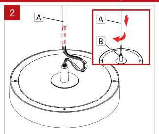
Pass the wires through the stem(A). Assemble the stem (A) into the cone (B) by screwing it.
