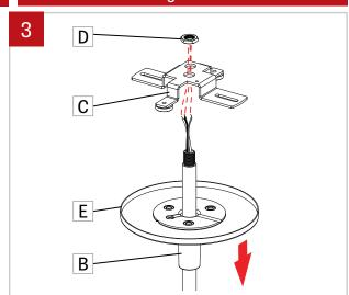
Pass the wires through the middle hole of the cross-bracket (C) and nut (D). Lower the canopy (E) and the cone (B) along the stem(C).
