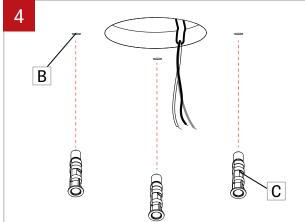
Remove the fixture. Drill the holes following the drill holes (B). Install the screw anchors (C). Recommended to have reinforcements on the back of the ceiling (wood recommended) where holes are drilled.
