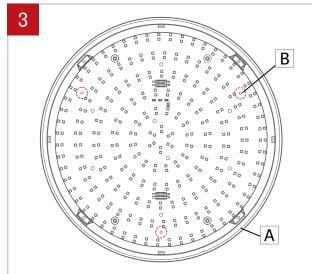
Use the fixture (A) as a model to mark 3 drill holes (B) on the ceiling.
