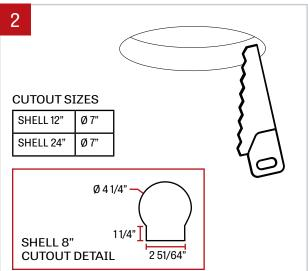
Prepare the area where the fixture is going to be installed. Cut the hole in the drywall ceiling.
