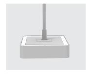
18" long x 1/2" diameter steel stem is available for all driver mounting options. Longer stems up to 48" are available. Stems cannot be cut in the field. Finished to match housing.
