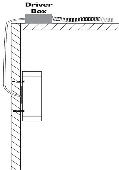
Driver is recessed with brackets for mounting to ceiling joists or other supporting members.
