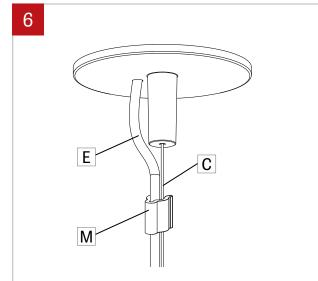
Secure the power cord(E) to the aircraft cable(C) with the plastic clip(M).
