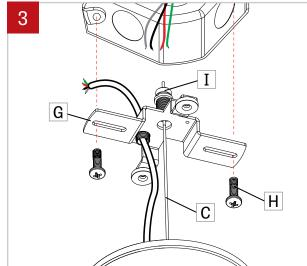
Install the cross-bracket(G) on the juction box with screws(H). Adjust the aircraft cable(C) length by pushing the feeder tube(I).
