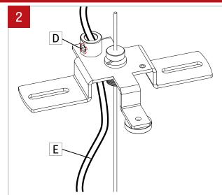
Tighten the srcrew(D) to secure the power cord(E) with the strain relif(F).
