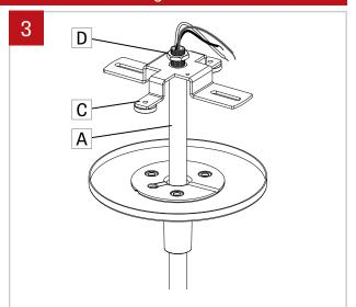
Install the cross-bracket (C) on the stem (A) by using the nut (D).
