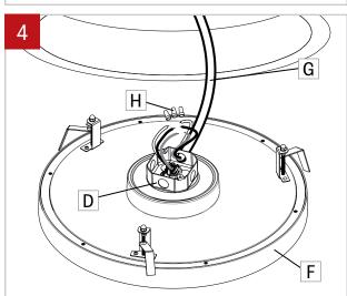
Make the electrical connection between the fixture (F) and main power cable (G) with marrettes (H) inside the junction box (D).
