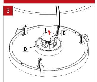
Open junction box (D) by removing junction box cover (E).
