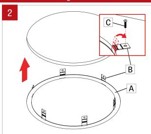
Install the ring (A) into the hole by bending the brackets (B) over the ceiling. Secure bent brackets with screws (C) on ceiling.
