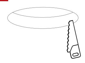
Prepare the area where the fixture is going to be installed. Cut the hole (24 1/16") in the drywall ceiling.
