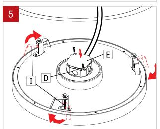
Close junction box (D) with junction box cover (E). Rotate the brackets (I) to stay above and inside of the fixture. Do not let the fixture hang by the wires.
