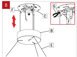
Pass the aircraft cables (E) through the canopy (B). Insert them into the grippers (F) then adjust the cables (E) by pushing the feeder tube (F). Cut the excess cable with an aircraft cable cutter (G). TOGO 36" and 48" have 4 wires.
