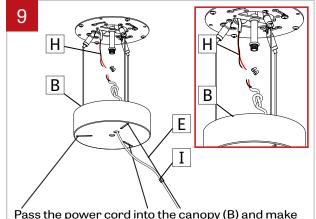
a knot. Make electrical connections between the power cord and remote driver feed (H). Installation may differ depending on your type of ceiling.
