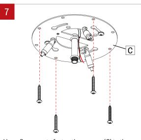
Use #8 screws to fasten the canopy (C) to the ceiling.
