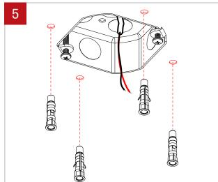
Remove the canopy plate and then drill holes (1/4"
