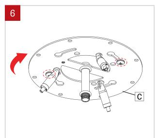
Tighten the two screws to secure the canopy (C) to the Junction box.
