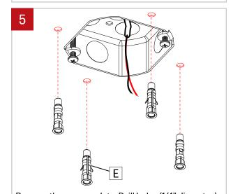
Remove the canopy plate. Drill holes (1/4" diameter) following the red marks. Install #8 screw anchors (E).
