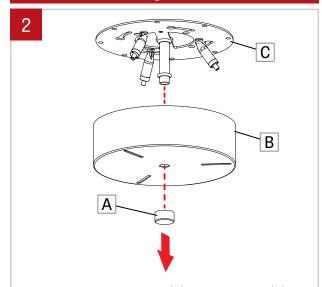
Loosen the decorative nut (A) on the canopy (B). Separate the canopy (B) from the canopy plate (C).
