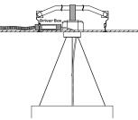
RDB - Ceiling Remote Driver for grid ceiling Driver is in a 20"x4"x2" enclosure with brackets for mounting to ceiling runners. The 5 1/2" diameter x 1 5/8" deep wiring compartment conceals and supports for suspension and power cables.
