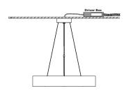
RDB - Drywall Remote Driver Driver is in a 20"x4"x2" enclosure with brackets for mounting to ceiling joists or other supporting members. The 51/2" diameter x15/8" deep wiring compartment canopy conceals and supports suspension and power cables. It is available in standard finishes (see ordering code).
