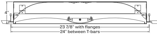
**VEGA - ST- screw slot t-bar**
