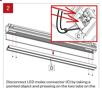
top. Unscrew the cartridge (D) and place it in a
