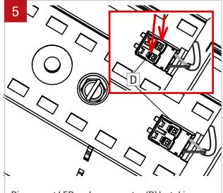
Disconnect LED molex connector (D) by taking a pointed object and pressing on the two tabs on the top.
