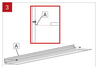
Locate the J-Bar (A) position using provided client drawing. Install wall bracket to wall. Align with structural stud or use drywall anchors when needed. For sleeve adjustment, please refer to end-sleeve installation sheet.
