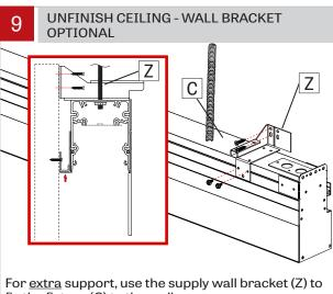
fix the fixture (C) to the wall.
