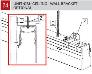
For <u>extra</u> support, use the supply wall bracket (Z) to fix the fixture (C) to the wall.
