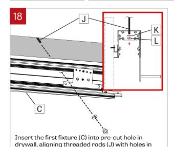
top of fixture (C). Put washers (K) and tighten nuts
