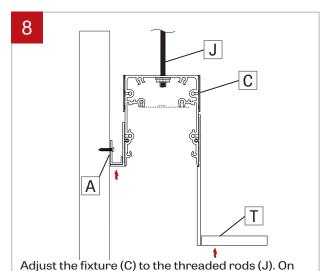
wall side, the fixture (C) must touch the J-Bar (A).
