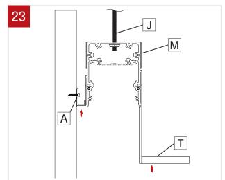
Adjust the second fixture (M) to the threaded rods (J). On wall side, the fixture (M) must touch the J-Bar (A). On ceiling side, flange need to be flush with the tile (T).
