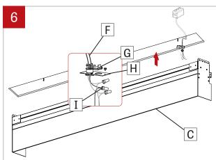
Install power cable (F) (by other) through the BX connector (G) (by other) and install onto the power plate (H) provided. Make electrical connections between power cable (F) and fixture cables using electrical marettes (I). Reinstall the power plate (H) to the fixture (C). Numbers of wires may vary.
