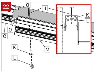
Insert the second fixture (M) into pre-cut hole in drywall, aligning threaded rods (J) with holes in top of fixture (M) and with the first fixture (C) with aligning brackets (O). Put washers (K) and tighten nuts (L) to secure the fixture (M).
