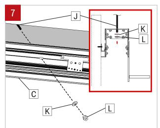
Insert fixture (C) into pre-cut hole in drywall, aligning threaded rods (J) with holes in top of fixture (C). Put washers (K) and tighten nuts (L) to secure the fixture (C).
