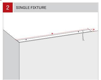
Prepare the area and mark the mounting point location where the fixture is going to be installed according to the dimensions [\*] in the client drawings.
