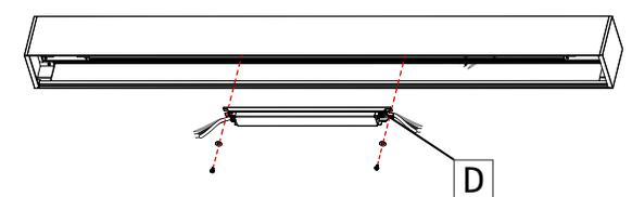
Unscrew the driver (D) from the fixture. Replace the driver and make connection with wire nuts.
