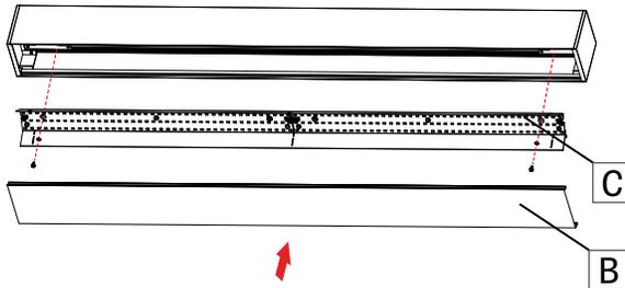
Reinstall the cartridges (C) by using a **screw with plastic washer (VIA 1.5-3-4-5)**. Do not apply too much pressure. Reconnect the wires to the LED boards correctly. Put the lens (B) back in place.
