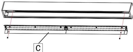
Unscrew the cartridge (C) and place it in a safe place.
