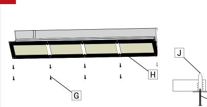
Fasten drywall screws (G) through the obround holes of the flanges (H).
