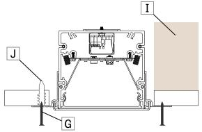
To reinforce the screws (G) that maintain the fixture in the drywall, wood blocking (I) or drywall anchors (J) must be used.
