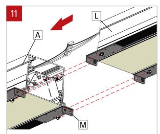
Slide the fixture (L) to the fixture (A), repeat for all sections in the run. Attach the two fixtures by fastening screws on the joiners (M).
