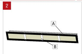
Make sure the power to the fixture (A) is turn off, the lens is installed on the fixture and protected by a cover. The spacer brackets (B) are in place, align with the obround holes of the flanges.
