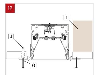
Fasten fixture to the ceiling by fastenning drywall screws (G) through flanges into anchors (J) of wood blocking (I).
