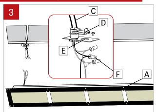
Install power cable (C) (by other) through the BX connector (D) (by other) and install onto the power plate (E) provided. Make electrical connections between power cable (C) and fixture cables using electrical marettes (F). Reinstall the power plate (E) to the fixture (A). Number of wires may vary.
