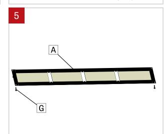
If the fixture position need adjustments, remove screws (G) on one side of the fixture (A) and adjust it. Reinstall the screws once the position is settled.
