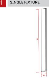
Prepare the area where the fixture is going to be installed. Cut hole in the drywall according to the dimensions [\*] given in the client drawings.
