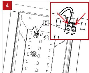
Disconnect LED molex connector (D) by taking a pointed object and pressing on the two tabs on the top.
