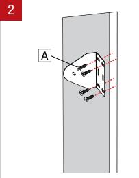
Insert mounting brackets (A) into the pre-cut hole and screw it to wall stud according to the dimensions given in the client drawings.
