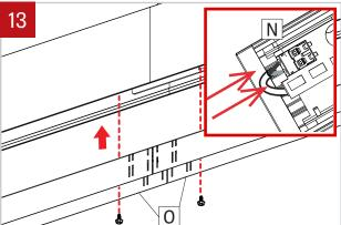
Reinstall the cartridge (0) and reconnect the LED molex connector (N). NOTE: connect black wire into the negative (-) terminal and the white wire into (+) positive terminal. Make sure that the wires are not hiding any LED diode. Screw the cartridge back in place by using screw with plastic washer. Do not apply too much pressure.
