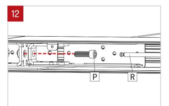
Join fixtures using align pins as guide. Put back in place the provided screw (P) (using 3/16" Ball-End Screwdriver (R) provided). Make sure that no wires are placed in between the extrusions, preventing the fixtures to be joined. Tight the screw (P) to pull the extrusions together. Repeat steps 10 to 12 for all others fixtures in the run.
