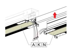
**2-** Slide the fixture **[N]** to the fixture **[A]**. Attach the two fixtures by fastening the screws on the joiners **[O]**.
