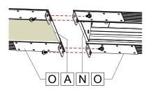
**3-** Raise the next fixture **[N]** and insert it in opening next to the previously mounted fixture **[A]**. Push wires **[Q]** of first fixture **[A]** into the next fixture **[N]**.
