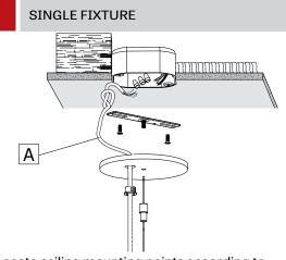
Locate ceiling mounting points according to supplied client drawing. Make a knot in the power cord (A) and then connect it to the ceiling power feed. Warning : Power must come from Single branch circuit.
