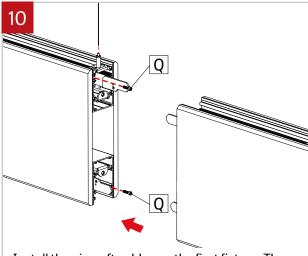
Install the aircraft cables on the first fixture. Then install it on the second fixture (as shown in steps 4 and 5). Remove the screw (Q) on the joiner and put it in a safe place.
