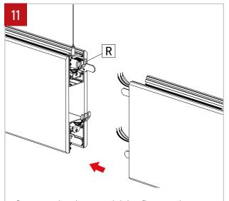
Connect wires between joining fixture using quick connectors (R). Number of wires may vary.
