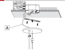
Locate ceiling mounting points according to supplied client drawing. Make a knot in the power cord (A) and then connect it to the ceiling power feed. Warning: Power must come from Single branch circuit.
