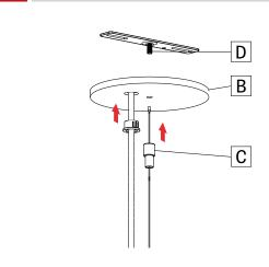
Secure canopy (B) with slip ring (C) on threaded rod (D).
