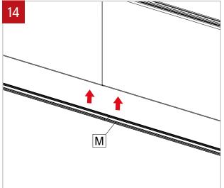
Re-install lens (M) by simply pushing in the lens until it snaps in . (push evenly to prevent from damaging the lens).
