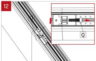
Join fixtures using align pins as guide. Put back in place the provided screw (Q) (using 3/16" Ball-End Screwdriver provided). Make sure that no wires are placed in between the extrusions, preventing the fixtures to be joined. Tight the screws (Q) on the top and bottom to pull the extrusions together. Repeat steps 10 to 12 for all others fixtures in the run.
