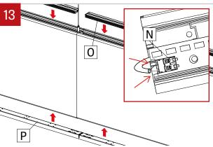
Reinstall the cartridge (O and P) and reconnect the LED molex connector (N). NOTE: connect blue wire into the negative (-) terminal and the red wire into (+) positive terminal. Make sure that the wires are not hiding any LED diode. Screw the cartridge (P) back in place by using screw with plastic washer. Do not apply too much pressure.
