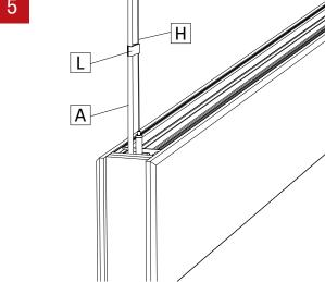
Secure power cord (A) to aircraft cable (H) with plastic clip (L).
