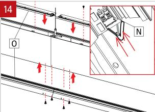
Replace the cartridges (O) and reconnect the LED molex connector (N). NOTE: connect black wire into the negative (-) terminal and the white wire into (+) positive terminal. Make sure that the wires are not hiding any LED diode. Screw the cartridge back in place.
