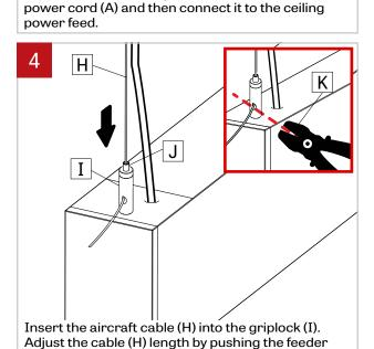
tube (J) and cut the excess cable with an aircraft
