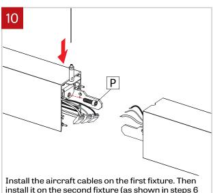
and 7). Remove the screw (P) on the joiner and put it
