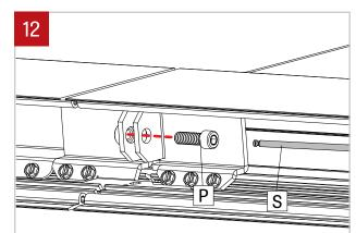
Join fixtures using align pins as guide. Put back in place the provided screw (P) (using 3/16" Ball-End Screwdriver (S) provided). Make sure that no wires are placed in between the extrusions, preventing the fixtures to be joined. Tight the screw (P) to pull the extrusions together. Repeat steps 13 to 15 for all others fixtures in the run.
