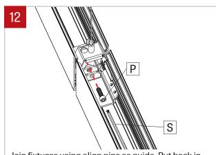
Join fixtures using align pins as guide. Put back in place the provided screw (P) (using 3/16" Ball-End Screwdriver (S) provided). Make sure that no wires are placed in between the extrusions, preventing the fixtures to be joined. Tight the screw (P) to pull the extrusions together. Repeat steps 10 to 12 for all others fixtures in the run.
