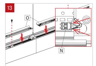
Replace the cartridge(s) (0) and reconnect the LED molex connector (N). **NOTE: connect black wire into** the negative (-) terminal and the white wire into (+) positive terminal. Make sure that the wires are not hiding any LED diode. Screw the cartridge back in place.
