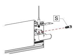
Align the second fixture **[T]** to the first fixture **[U]**. Join the fixtures together. Put the joiner screw **[S]** back and tighten using a 3/16" ball-end screwdriver **[V]** to pull the extrusions together.
