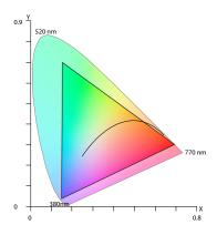
The above diagram overlays the full gamut of colors attainable with the RGBW on top of the CIE 1931 color space. Any color point inside of the triangle can be obtained by setting the correct output levels for each of the individual red, green, blue, and white channels.
