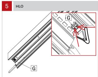
Disconnect LED molex connector (G) by taking a pointed object and pressing on the two tabs on the top.
