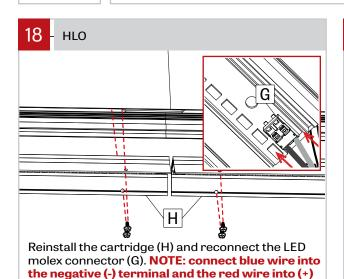
positive terminal. Make sure that the wires are not hiding any LED diode. Screw the cartridge back in
