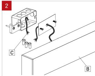
Make wire connection between fixture (B) and wall power cable (C). Number of wires may vary.
