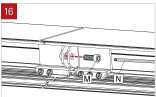
Join fixtures using align pins as guide. Put back in place the provided screw (M) (using 3/16" Ball-End Screwdriver (N) provided). Make sure that no wires are placed in between the extrusions, preventing the fixtures to be joined. Tight the screw (M) to pull the extrusions together. Repeat steps 9 to 12 for all other fixture. Then tighten all screws on mounting brackets.
