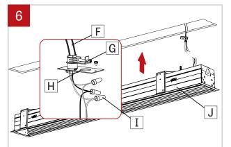
Install power cable (F) (by other) through the BX connector (G) (by other) and install onto the power plate (H) provided. Make electrical connections between power cable (F) and fixture cables using electrical marettes (I). Reinstall the power plate (H) to the fixture (J). Insert the fixture into pre-cut hole in drywall. Number of wires may vary.
