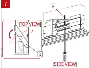
Tighten the drywall bracket screws (E) to rotate the drywall brackets (D) in place. Tighten the drywall bracket screws (E) to lock into place.
