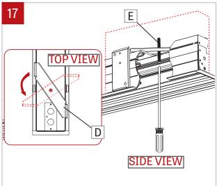
Tighten the drywall bracket screws (E) to rotate the drywall brackets (D) in place. Tighten the drywall bracket screws (E) to lock into place.
