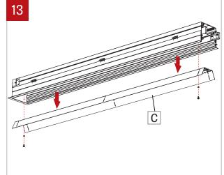
Remove all the end LED cartridges (C).
