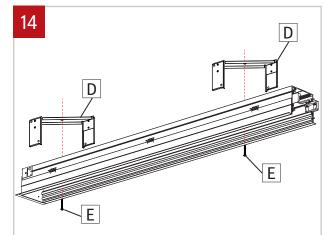
Remove the screw (E) from the drywall bracket (D). Install the drywall brackets (D) on the fixture and secure them by putting back in place the screws (E). Make sure that the screws are not overtighten and that the drywall brackets (D) don't rotate in place.
