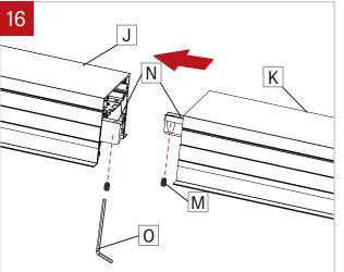
Slide the fixture (J) to the fixture (K) using alignment pins as guides. Tighten the set screws (M) on both joigning brackets (N) using an Allen Key (O) to secure the fixtures together.
