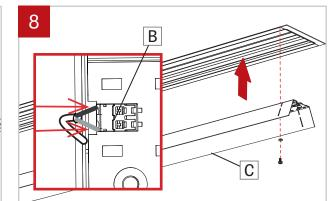
Reinstall the cartridge(s) (C) and reconnect the LED molex connector (B). **NOTE: connect black wire into the negative (-) terminal and the white wire into (+) positive terminal.** Make sure that the wires are not hiding any LED diode. Screw the cartridge back in place by **using screw with plastic washer. Do not apply too much pressure.**
