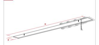
Prepare the area where the fixture is going to be installed. Cut hole in the drywall according to the dimensions [\*] in the client drawings.
