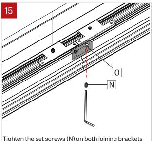
(0) using Allen Key to secure the fixtures together.
