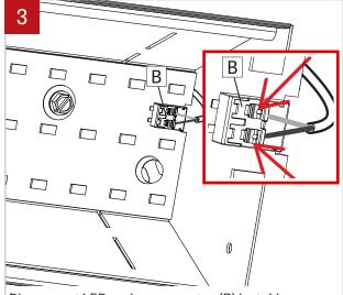
Disconnect LED molex connector (B) by taking a pointed object and pressing on the two tabs on the top.
