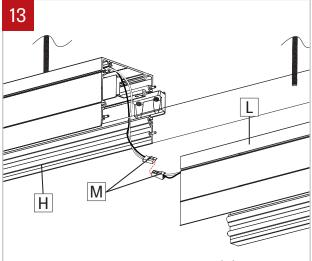
Apply steps 5 and 6 to the first fixture (H) in the run. Make wires connection between fixture (H) and (L) using quick connectors (M).
