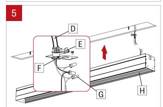
Install power cable (D) (by other) through the BX connector (E) (by other) and install onto the power plate (F) provided. Make electrical connections between power cable (D) and fixture cables using electrical marettes (G). Reinstall the power plate (F) to the fixture (H). Number of wires may vary.
