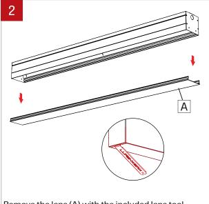
Remove the lens (A) with the included lens tool.
