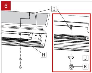
Insert fixture (H) into pre-cut hole in drywall, aligning threaded rods (I) with holes in top of fixture (H). Put washers (J) and tighten nuts (K) to secure the fixture (H).
