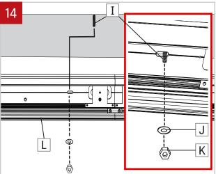
Insert the second fixture (L) into pre-cut hole in drywall, aligning threaded rods (I) with holes in top of fixture (L). Put washers (J) and tighten nuts (K) to secure the fixture (L).
