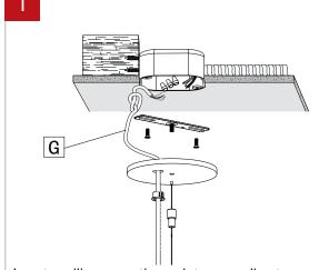
Locate ceiling mounting points according to supplied client drawing. Make a knot in the power cord (G) and then connect it to the ceiling power feed.
