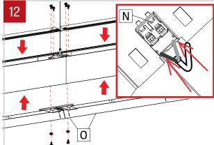
Reinstall the cartridges (O) and reconnect the LED molex connector (N). NOTE: connect black wire into the negative (-) terminal and the white wire into (+) positive terminal. Make sure that the wires are not hiding any LED diode. Screw the cartridge back in place by using screw with plastic washer (for direct only). Do not apply too much pressure.
