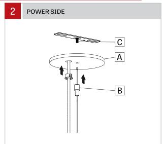
Secure canopy (A) with slip ring (B) on threaded rod (C).
