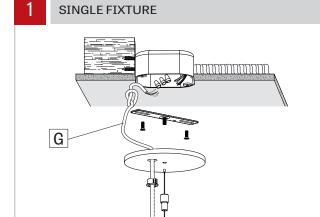
Locate ceiling mounting points according to supplied client drawing. Make a knot in the power cord (G) and then connect it to the ceiling power feed.
