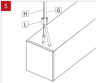
Secure power cord (G) to aircraft cable (H) with plastic clip (L).
