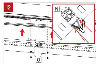
Reinstall the cartridges (O) and reconnect the LED molex connector (N). NOTE: connect black wire into the negative (-) terminal and the white wire into (+) positive terminal. Make sure that the wires are not hiding any LED diode. Screw the cartridge back in place by using screw with plastic washer. Do not apply too much pressure.
