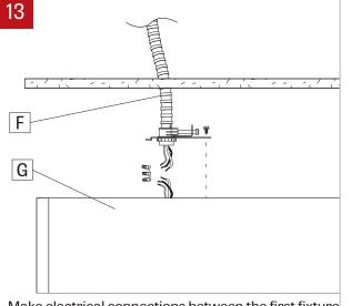
Make electrical connections between the first fixture (G) and main power (F).
