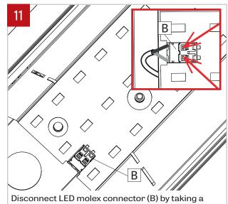
Disconnect LED molex connector (B) by taking a pointed object and pressing on the two tabs on the top.
