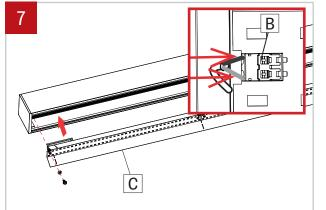
Reinstall the cartridge (C) and reconnect the LED molex connector (B). **NOTE: connect black wire into the negative (-) terminal and the white wire into (+) positive terminal.** Make sure that the wires are not hiding any LED diode. Screw the cartridge back in place by **using screw with plastic washer. Do not apply too much pressure.**
