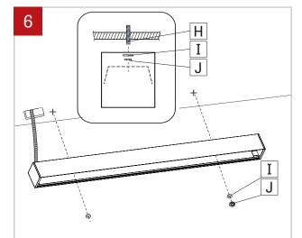
Fasten fixture to threaded stud (H) using washer (I) and nuts (J). (If there's no threaded stud present, the fixture can be screwed directly onto the ceiling).
