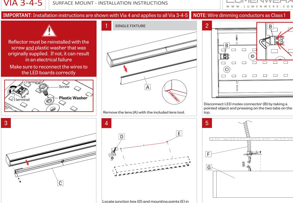
Make electrical connections between main power (F) and fixture (G). Number of wires may vary.
