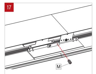
Join fixtures together and Secure them together with supplied screws (M). Repeat steps 15 to 17 for all other fixture. Then tighten all washers and nuts on threaded studs to secure the fixtures.
