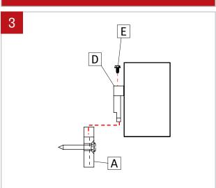
Insert fixture bracket (D) into wall bracket (A), and secure in place with suplied screws (E).
