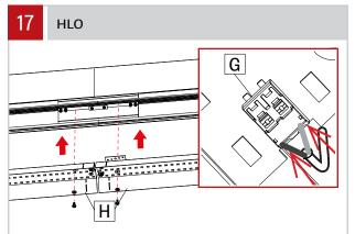
Reinstall the cartridge(s) (H) and reconnect the LED molex connector (G). **NOTE: connect the blue wire into negative (-) terminal and the red wire into (+) positive terminal.** Make sure that the wires are not hiding any LED diode. Screw the cartridge back in place by using screw with plastic washer. Do not apply too much pressure.
