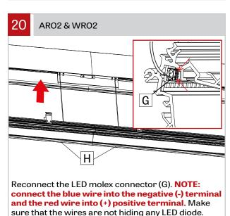
Reinstall the cartridge (H) back in place.
