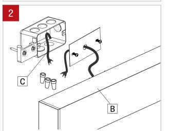
Make wire connection between fixture (B) and wall power cable (C). Number of wires may vary. Warning: Power must come from Single branch circuit
