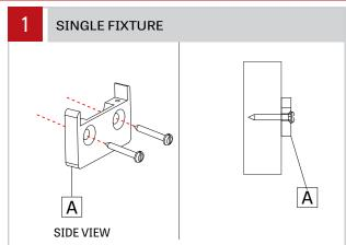
Locate wall bracket position using provided client drawing. Install mounting brackets (A) to wall. Align with structural stud (need double studs distance between screws is 1.250"). Flat head Philips drive screw, nominal size #10, min. length 1.250".
