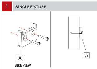
Locate wall bracket position using provided client drawing. Install mounting brackets (A) to wall. Alian with structural stud (need double studs distance between screws is 1.250"). Flat head Philips drive screw, nominal size #10, min. length 1.250".
