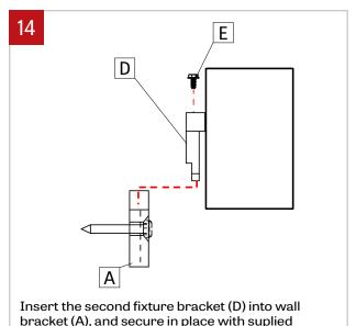
screws (E). Do not overtighten.
