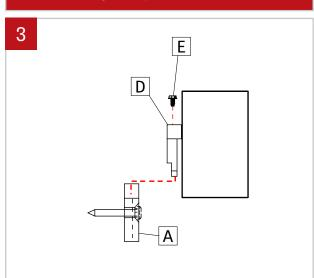
Insert fixture bracket (D) into wall bracket (A), and secure in place with suplied screws (E).
