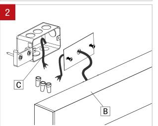
Make wire connection between fixture (B) and wall power cable (C). Number of wires may vary. Warning: Power must come from Single branch circuit
