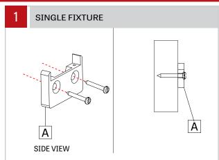
Locate wall bracket position using provided client drawing. Install mounting brackets (A) to wall. Align with structural stud (need double studs - distance between screws is 1.250"). Flat head Philips drive screw, nominal size #10, min. length 1.250".
