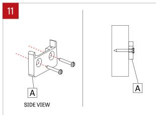
Locate wall bracket position for the second fixture using provided client drawing. Install mounting brackets (A) to wall. Align with structural stud (need double studs - distance between screws is 1.250"). Flat head Philips drive screw, nominal size #10, min. length 1.250".
