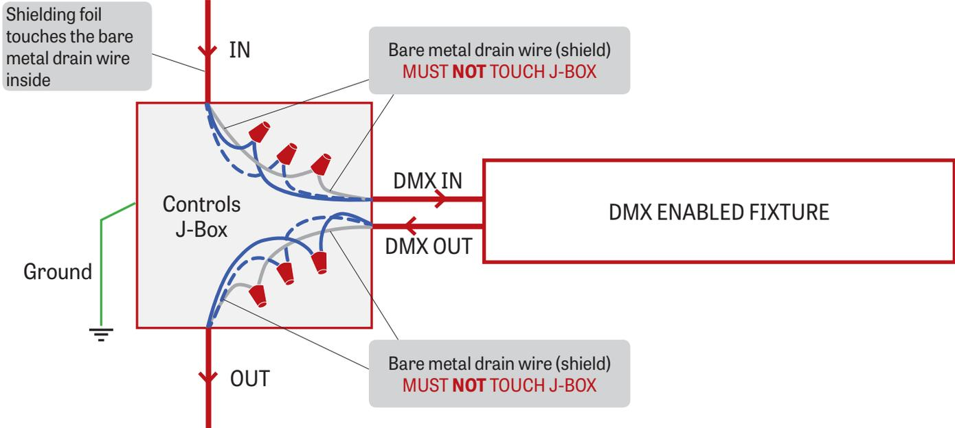
Low capacitance DMX cable to next fixture
