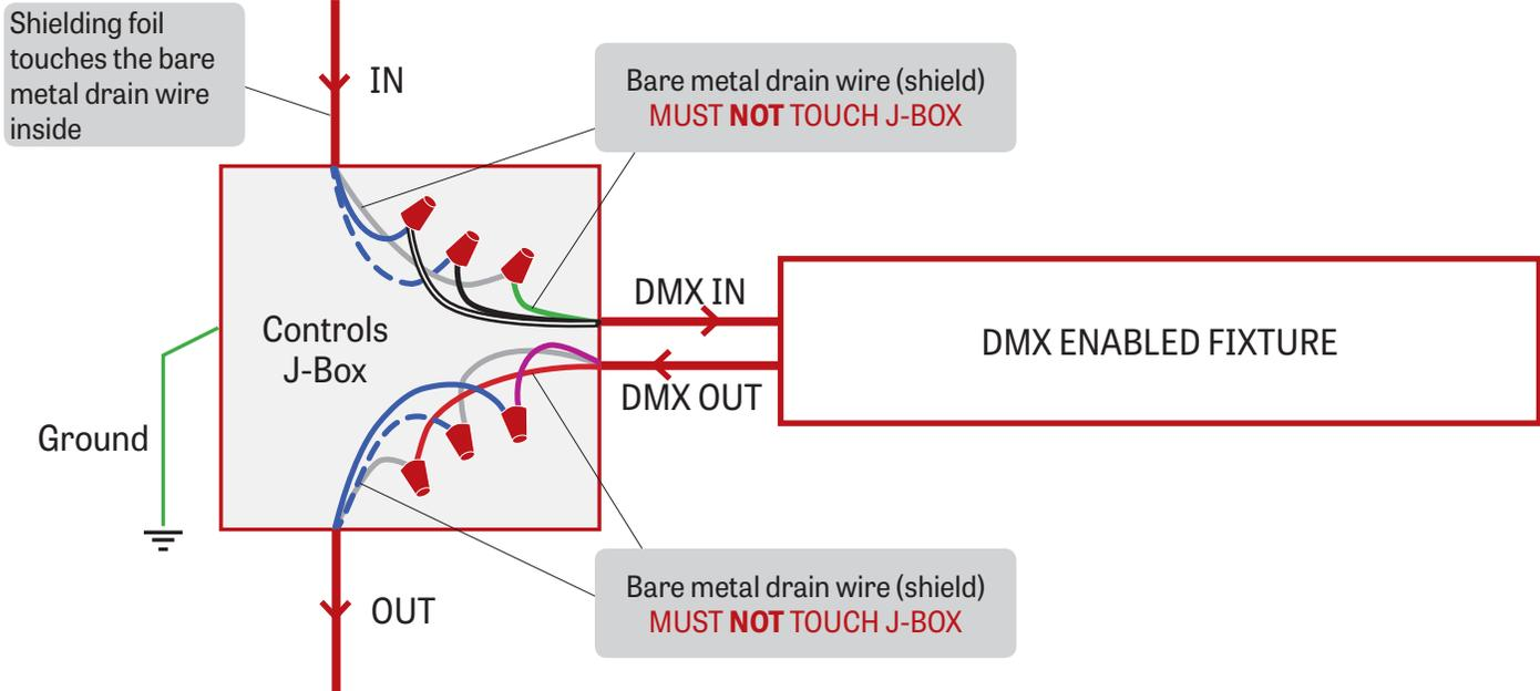
Low capacitance DMX cable to next fixture
