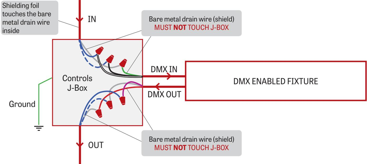
Low capacitance DMX cable to next fixture
