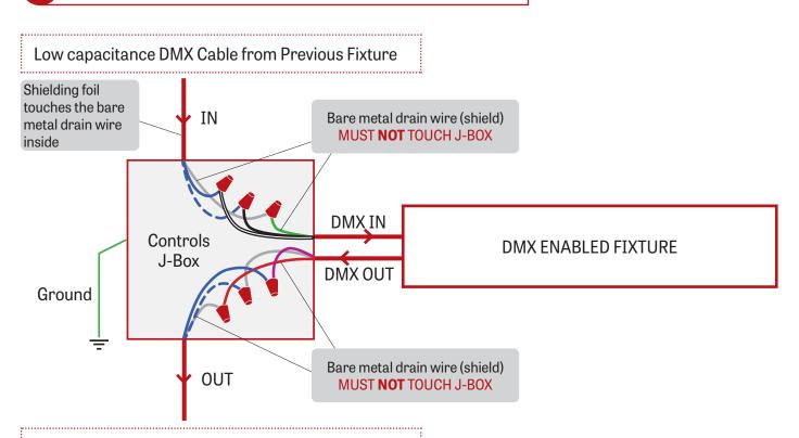
Low capacitance DMX cable to next fixture
