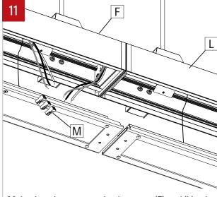
Make the wires connection between (F) and (L) using quick connectors (M). Numbers of wires may vary.
