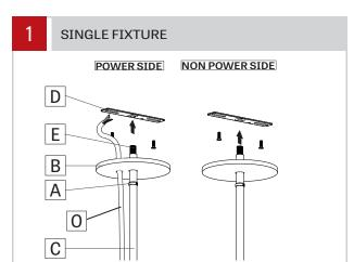
Make sure that the power to the fixture is turned off. Slide the slip ring (A) and the canopy (B) onto the stem (C) and leave some space. Screw the junction box crossbar (D) with the threaded rods (E) onto the stem (C). Wet-location power-cord is supplied by us (O).
