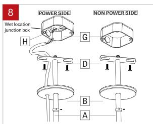
Raise the first fixture and tighten the junction box crossbars (D) with screws to the junction boxes (G). Make wire connection on the power side with wire connectors (H). Then slide the canopies (B) and thighten the sets up with the slip rings (A).
