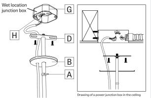
Raise the fixture and tighten the junction box crossbar (D) with screws to the junction box (G). Make wire connection with wire connectors (H). Then slide the canopy (B) and thighten the set up with the slip ring (A).
