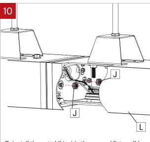
Reinstall the nuts (J) inside the second fixture (L) on the joiner to secure it.
