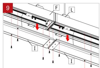
Push the wires of the second fixture (L) inside the first fixture (F) through the holes of the end caps. Align the second fixture (L) to the screws of the joiner of the first fixture (F). Attach the second fixture (L) to the ceiling as shown in step 8. Unscrew and lower the lens frames (I) of the two fixtures retained by security cables.
