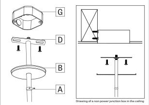
Raise the fixture and tighten the junction box crossbar (D) with screws to the junction box (G). Then slide the canopy (B) and thighten the set up with the slip ring (A).
