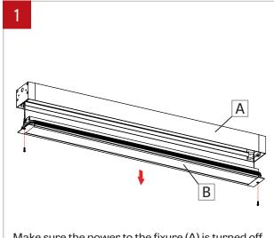
Make sure the power to the fixure (A) is turned off. Unscrew and lower the lens frame (B) retained by security cables.
