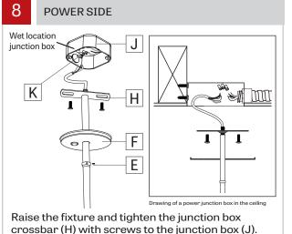
Make wire connection with wire connectors (K).
