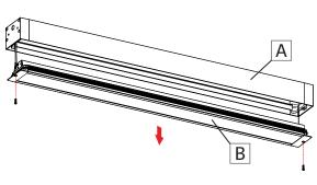
Make sure the power to the fixure (A) is turned off. Unscrew and lower the lens frame (B) retained by security cables. Fixture must be installed with lens facing down.
