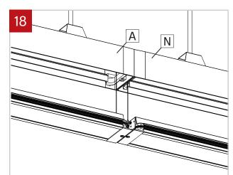
Push the wires of the second fixture (N) inside the first fixture (A) through the holes of the end caps. Align the second fixture (N) to the screws of the joiner of the first fixture (A). Attach the second fixture (N) to the ceiling as shown in step 17.
