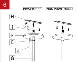
Slide the slip ring (E) and the canopy (F) onto the stem (G) and leave some space. Screw the junction box crossbar (H) with the threaded rods (I) onto the stem (G). Wet-location power-cord is supplied by us (J).
