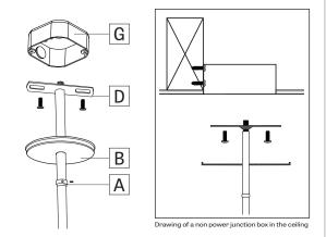
Raise the fixture and tighten the junction box crossbar (D) with screws to the junction box (G). Then slide the canopy (B) and thighten the set up with the slip ring (A).
