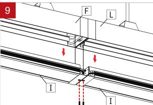
Push the wires of the second fixture (L) inside the first fixture (F) through the holes of the end caps. Align the second fixture (L) to the screws of the joiner of the first fixture (F). Attach the second fixture (L) to the ceiling as shown in step 8. Unscrew and lower the lens frames (I) of the two fixtures retained by security cables.
