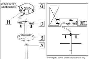
Raise the fixture and tighten the junction box crossbar (D) with screws to the junction box (G). Make wire connection with wire connectors (H). Then slide the canopy (B) and thighten the set up with the slip ring (A).
