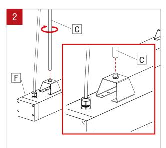
Screw the stems (C) onto the nipple at the ends of the fixture (F).  $\,$
