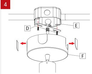
Fix the Cross bar (D) to the Junction box (E) using screws. Punch out the knock outs of the Canopy (F) to allow the conduits to fit.
