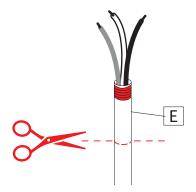
Adjust the cable length by cutting and stipping the fixture cable (E) to the desire length for the height of the fixture. Reconnect the cables to the driver once adjustment is made.
