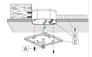
Connect the Main Power Quick Connect (A) to the BX cable (B). Secure Universal Crossbar (C) onto the Junction box (D).
