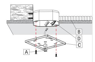
Connect the Main Power Quick Connect (A) to the BX cable (B). Secure Universal Crossbar (C) onto the Junction box (D).
