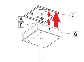
Connect the Fixture Quick Connect (F) to the Main power Quick Connect (A). Secure the Canopy (G) onto the Universal Crossbar (C).
