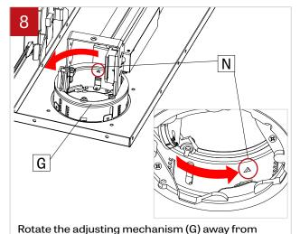
driver to have easier access. Opening (N) is aligned
