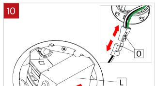
For Type-IC, pull out driver (L) from opening.
