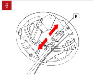
Disconnect the quick connectors (K) between the light element and the driver.
