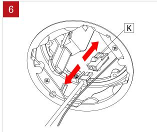
Disconnect the quick connectors (K) between the light element and the driver.
