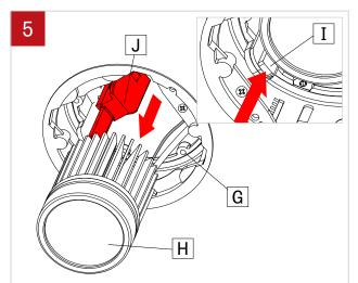
Push tab (I) on the side of the light element (H) to release it from the adjusting mechanism (G). Slide light element (H) from the track system (J).
