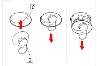
For trimless wall wash installation, detach baffle (C) by using provided suction tool (D). Stick tool on baffle lens and pull.
