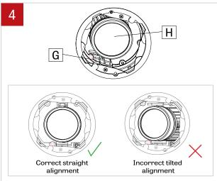
Straighten light element (H) by rotating and tilting the adjusting mechanism (G) to allow its removal in the next step.
