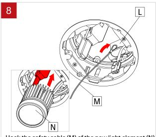
Hook the safety cable (M) of the new light element (N) to the driver (L).
