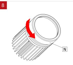
Unscrew lens cover (N) from heatsink of light element.
