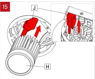
Insert light element (H) through track system (J). For standard depth, install until first click. For deep regressed depth, install until secondary click.
