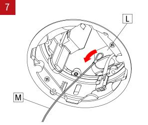
Pull the driver (L) towards the opening. Unhook safety cable (M) of light element from driver (L). Safely store light element on the side.
