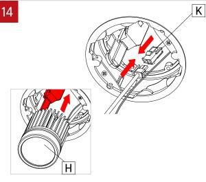
Reconnect light element (H) to driver with quick connectors (K).
