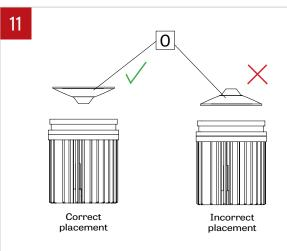
Make sure to position new optic (O) with flat surface facing outwards.
