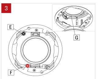
Slightly unscrew white screw (E) and red screw (F) located inside to allow rotation of the adjusting mechanism (G).
