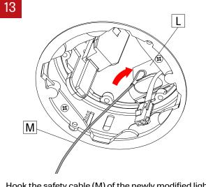
Hook the safety cable (M) of the newly modified light element to the driver (L).
