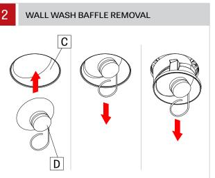
For trimless wall wash installation, detach baffle (C) by using provided suction tool (D). Stick tool on baffle lens and pull.
